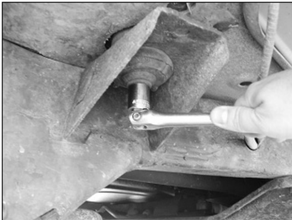
(Fig 1) Remove Factory Body Mount Bolt
