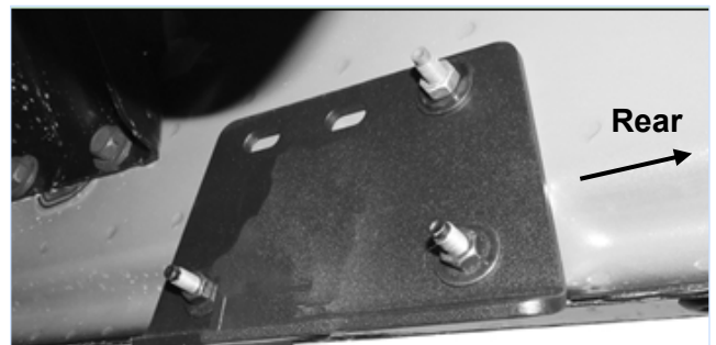
(Fig 3) Passenger Front Side with Mounting Bracket Installed
