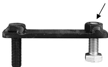
(Fig 3) Thread (1) M8X1.25-30 Hex Bolt into the nut on the plate. Stop when bolt reaches end of nut as pictured)
