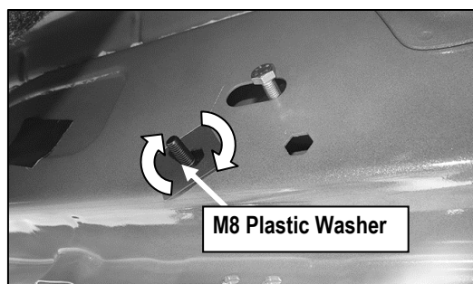
(Fig 5) Thread Plastic Washer onto Bolt Plate to hold Bolt/Nut Plate in position
