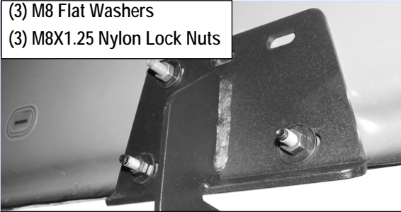
(Fig 7) Passenger Rear Side with Mounting Bracket Installed
